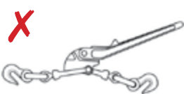
No over-center lever load binders (Dogs)
