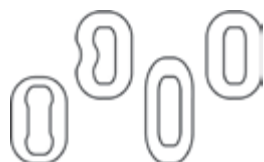
Chains with elongated, worn or bent links must not be used for restraint
