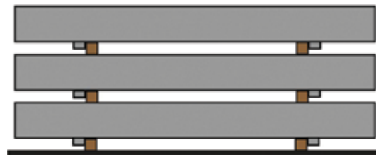
Both pieces of dunnage located outside the barrier feet
