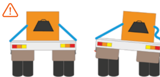
Small building movements are expected during transit resulting in chain slack, cable ties will prevent load binder hooks becoming detached from the chain
