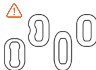
Chains with elongated, worn or bent links must not be used for restraint
