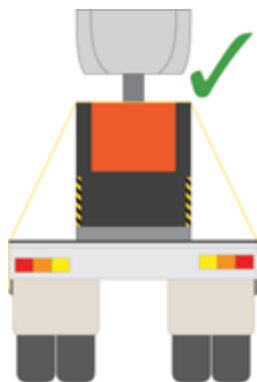
Load single file light cube centrally across the deck
