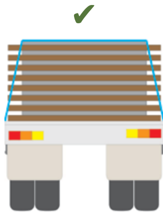
Load single file Shoring plate centrally across the deck.
