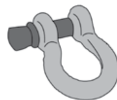
Bow shackles rated to 4 x lashing capacity of chain. Maximum of 2 chains.
