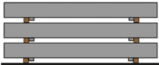
Both pieces of dunnage located inside the barrier feet
