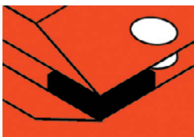
Rubber matting between shoring boxes
