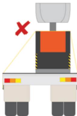
Do not load single file light cubes to one side
